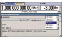
▲ Fig. 3 Emulation mode: Sample selection of a legacy signal generator to be emulated – example shown here is the R&S SMA 100A.
