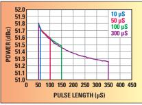
Arr Fig. 5 Output power vs. time,  $V_{DD} = 40 \text{ V}$ ,  $P_{IN} = 41 \text{ dBm}$ , duty cycle = 10%.
