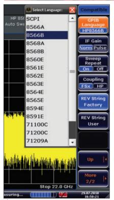
Fig. 2 Emulation mode: Selection of legacy signal analyzers to be emulated by the R&S FSV.
