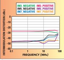
ightharpoonup Fig. 3 Intermodulation distortion performance vs. tone spacing,  $V_{DD} = 40 \text{ V}$ , frequency = 8.2 GHz, output power = 43 dBm/20 W.
