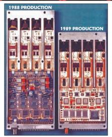
Fig. 3 Early U.S. developed quad T/R module technology.
