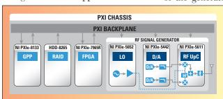
▲ Fig. 1 Example of a modular RF instrumentation system.
