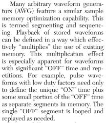
Many different waveform segments can be stored in the AWG waveform memory. Sequences are formed, using a contiguous series of segments. Because each segment has a specified start and stop address, sequence play is continuous and without gaps, when played from one segment to the next. Multiple segments can be grouped and looped for even greater memory compression. This waveform scenario construction is illustrated in *Figure 3*.
