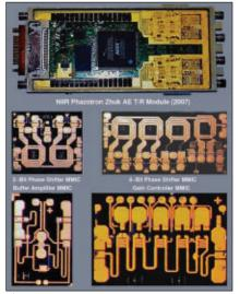
Fig. 2 Phazotron Zhuk AE X-Band quad module and MMIC chips.
