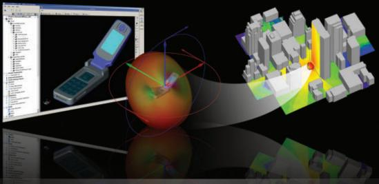
Cell phone antenna simulation in **XFdtd**
