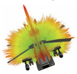
RCS & Surface Current Simulation of a Helicopter
