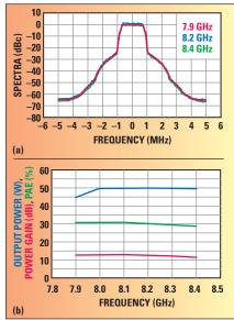
▲ Fig. 2 CGHV96100F1 typical performance spectral mask under OQPSK modulation, 1.6 Msps  $V_{\rm DD} = 40$  V, output power = 47 dBm/50 W (a) and linear output power, gain and PAE,  $V_{\rm DD} = 40$  V,  $I_{\rm DQ} = 1000$  mA, 1.6 Msps, OQPSK modulation at –30 dBc (b).
