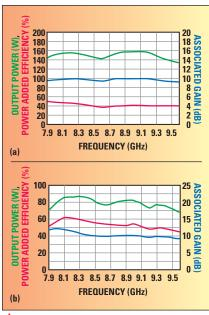
Fig. 4 CGHV96100F2: 100 W X-Band internally matched transistor (a) and CGHV96050F2: 50 W X-Band internally matched transistor (b) performance.
