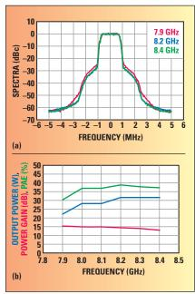
▲ Fig. 1 CGHV96050F1 typical performance spectral mask under OQPSK modulation, 1.6 Msps  $V_{\rm DD} = 40~V$ , output power = 44 dBm/25 W (a) and linear output power, gain and PAE,  $V_{\rm DD} = 40~V$ ,  $I_{\rm DQ} = 500~mA$ , 1.6 Msps, OQPSK modulation at −30 dBc (b).
